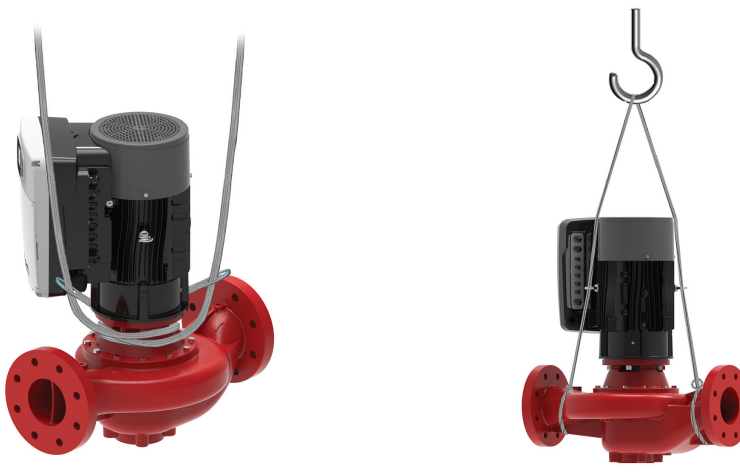
Acceptable lifting methods for close-coupled end-suction models e-1531X and e-1532X
