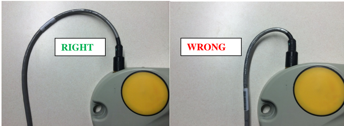
Figure 58. When installing an SL, it is always best to keep the cable STRAIGHT as it comes out the back of the instrument to keep debris from snagging on the cable. However, if the cable needs to be bent, keep the bend radius at 4 in (10 cm) or larger to avoid stress on the cable over time.
