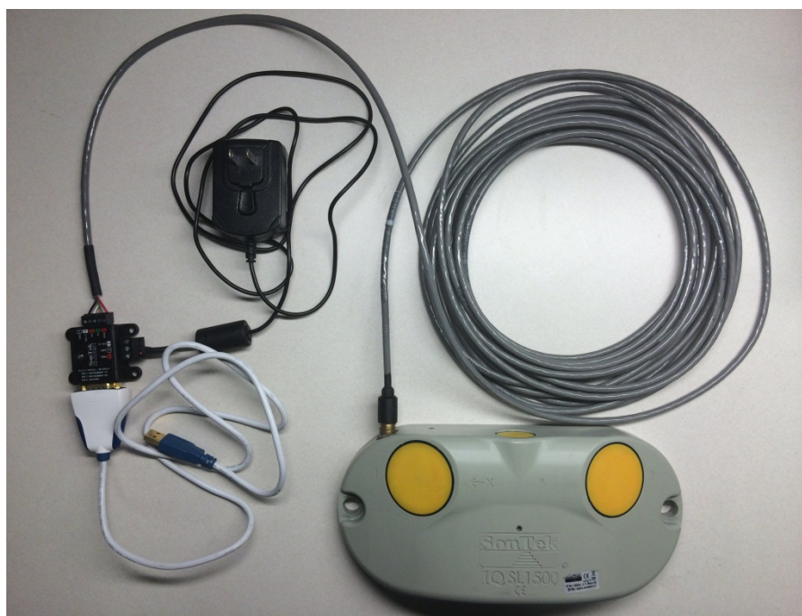
Figure 13. Connecting the USB-Serial adaptor to cable adaptor
