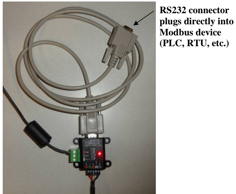
Figure 83. Connect to Modbus network using the RS232 cable
