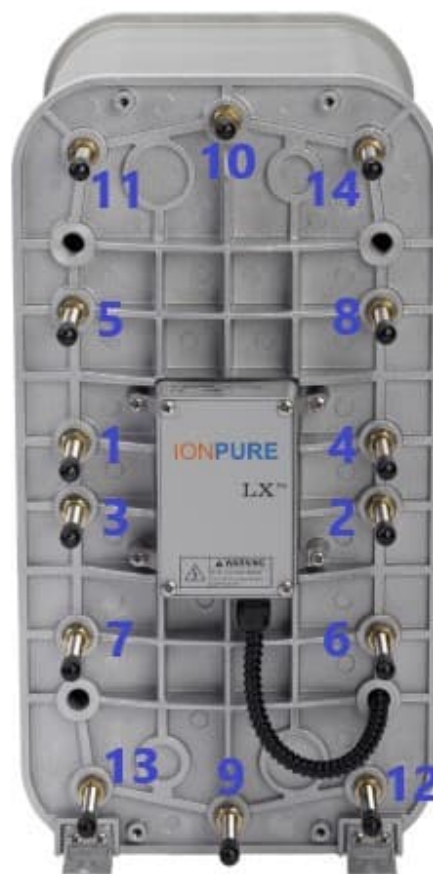
Figure 3-2 LX Tightening Sequence
