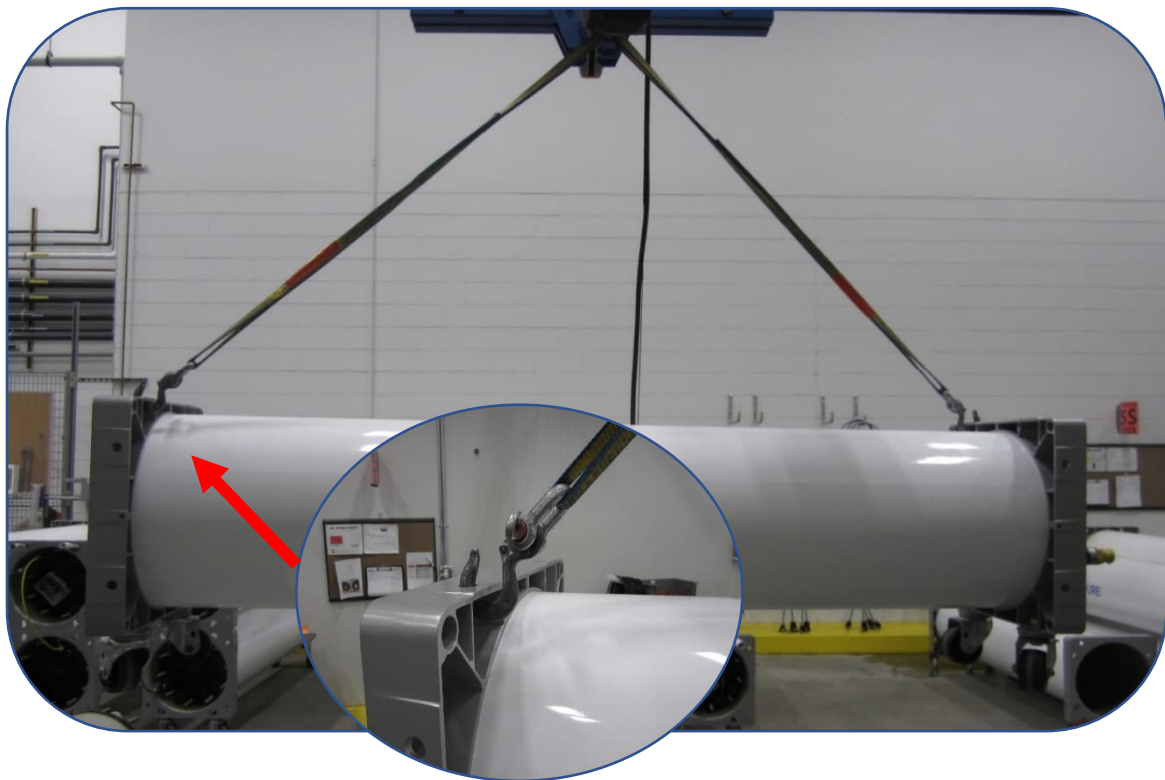
Figure 2-1: Lifting VNX module via housing FlexMounts
