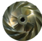
5-axis, CNC-milled aluminum alloy impeller with an anodized coating
