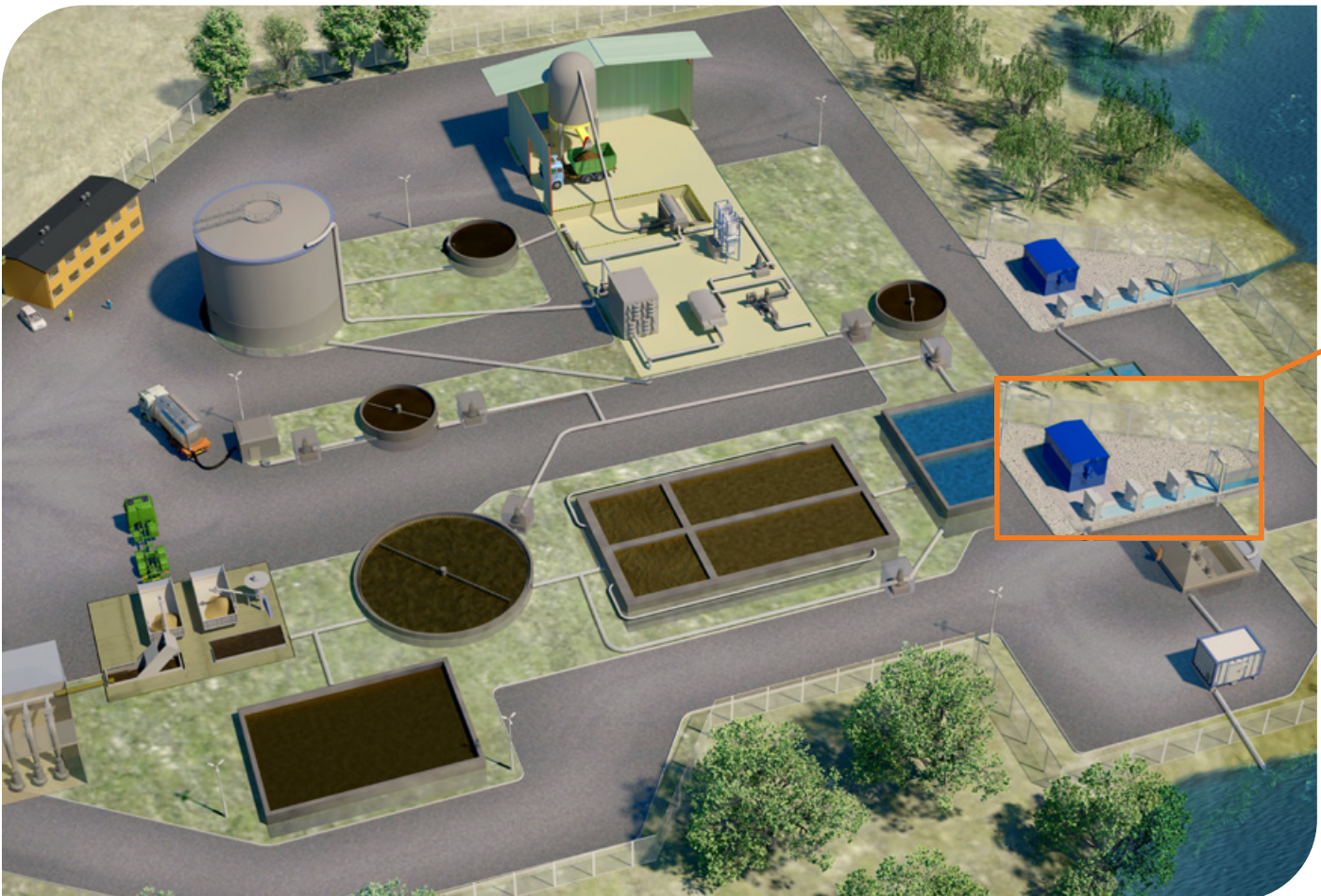
Schematic of a typical wastewater treatment facility incorporating a WEDECO brand TAK 55 UV system as a final treatment stage.
